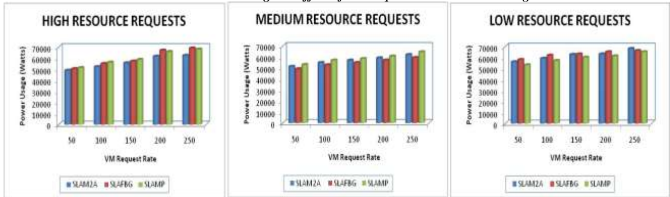
Fig 16: Effect of VM request Rate on Power Usage
